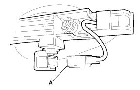
11. Pull the outer handle (A) out, and back as shown to remove it from the door. Take care not to scratch the door.
