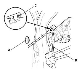
7. Driver's door: While holding the flange portion (A) of the outer casing cover (B), pull out the retainer (C), and pull the lock cylinder cable (D) away from the latch actuator (E).
