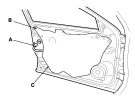
4. Pull the glass run channel (A) away as needed, and remove the bolt, then remove the center lower channel (B) by pulling it downward.
