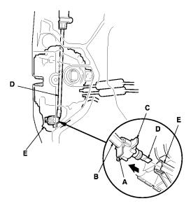
8. While holding the outer handle cover (A) from out side of the door, loosen the bolt, and then release the hooks (B) of the outer handle cover, then remove the cover and the lock cylinder (C) (driver's door) or the outer handle holder (passenger's door) from the outer handle base (D).
