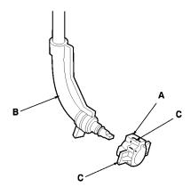
10. Disconnect the outer handle light connector (A).
