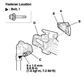
9. If the retainer (A) of the lock cylinder cable (B) is damaged, release the hooks (C), then replace it.
