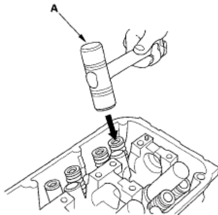
Fig. 128: Tapping End Of Valve Stem With Plastic Mallet Courtesy of AMERICAN HONDA MOTOR CO., INC.
