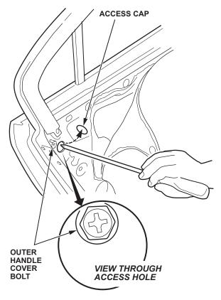
10. While holding the outer handle cover from the outside of the door, loosen the bolt. Pull back on the cover to release its hooks from the outer handle base.
