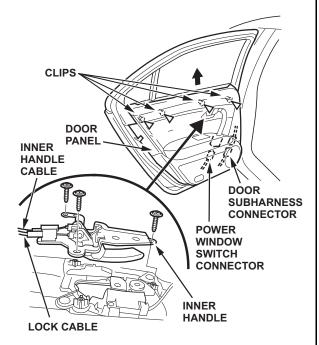
6. Using a clip remover, remove the remaining clips from the door. Using a knife, cut the bosses off the clips. Push each clip, then pull it away.
