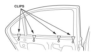
7. Peel back the upper left corner of the plastic inner door cover.
