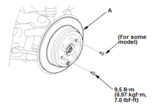
1. Install the brake disc/drum (A).
