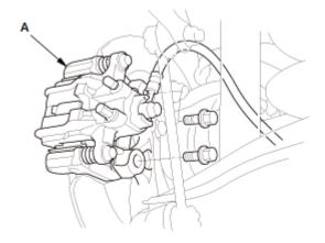
1. Remove the caliper assembly (A).
