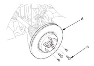
NOTE: If the brake disc is stuck to the front hub, thread two 8 x 1.25 mm bolts (B) into the brake disc to push it away from the front hub. Turn each bolt 90 degrees at a time to prevent the brake disc from binding.
