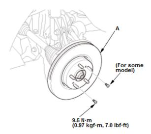
1. Install the brake disc (A).
