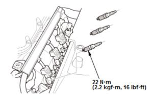
1. Apply a small amount of anti-seize compound to the plug threads, and screw the plugs into the cylinder head, finger tight, then tighten the plugs to the specified torque.
