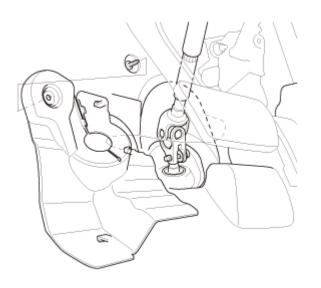
7. Steering Column Lower Slide Shaft - Hold
