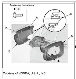
1. Release the hooks (A, B), then remove the visor (C) and the mirror housing (D).
