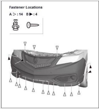
1. Remove the clips (A) and the screws (B).
