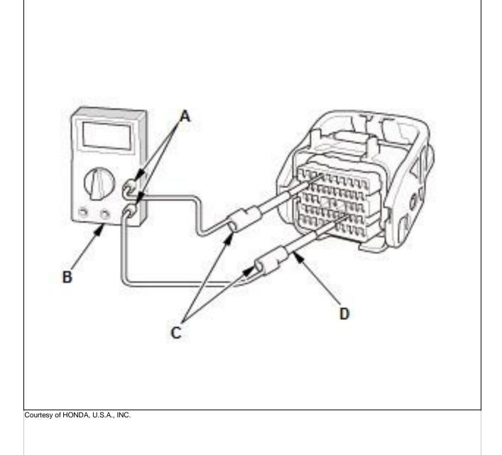
6. Gently contact the pin probe (male) at the terminal test port from the terminal side. Do not force thetips into the terminals.
