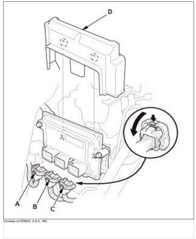
3. Disconnect PCM connectors A, B, and C.
