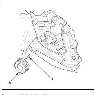
1. Remove the timing belt drive pulley (A) and the key (B).
