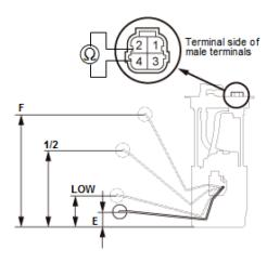
Measure the resistance between fuel tank unit 4P connector terminals No. 2 and No. 4 with the float at E (EMPTY), LOW (LOW FUEL INDICATOR), 1/2 (HALF FULL), and F (FULL) positions. If you do not get the following readings, replace the fuel gauge sending unit.
