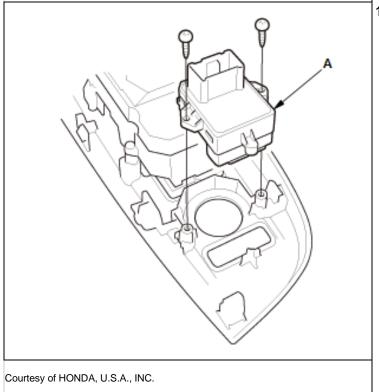
1. Install the power mirror switch (A).
