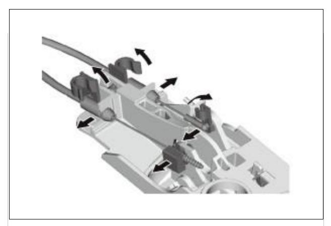
4. Front Door Armrest/Power Window Switch Panel - Remove (Driver's Side)
