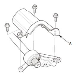
1. Remove the heat shield (A).
