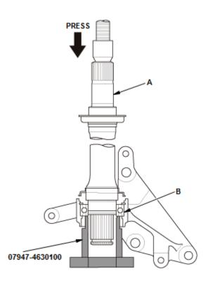
1. Press the intermediate shaft (A) into the shaft bearing (B) using the 39.2 x 49.5 x 15 mm fork seal driver and a press.
