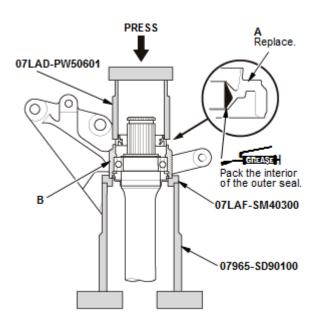
1. Install a new outer seal (A) into the bearing support (B) using the 40 mm installer attachment, the support base attachment, the support base, and a press. Press in the seal until it is even with the surface of the bearing support.
