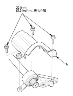
1. Install the heat shield (A).
