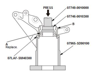
2. Press the intermediate shaft bearing (A) out of the bearing support (B) using the 15 x 135L driver handle, the 42 x 47 mm bearing driver attachment, the support base attachment, the support base, and a press.
