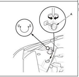
6. If adjustment is necessary, open the hood and adjust the headlights to local requirements by turning the adjuster (A).
