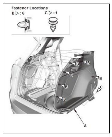
5. Remove the rear seat-back release lever/cable (A).
