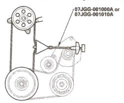
2. If you installed a new belt, run the engine for 5 minutes, then readjust the belt to the used belt specifications.
