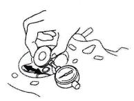
3. Subtract the O.D. of the valve stem, measured with a micrometer, from the I.D. of the valve guide, measured with an inside micrometer or ball gauge. Take the measurements in three places along the valve stem and three places inside the valve guide. The difference between the largest guide measurement and the smallest stem measurement should not exceed the service limit.
