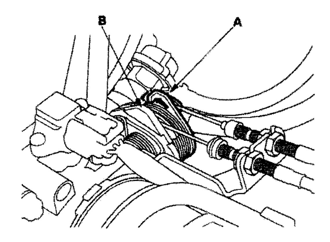
3. Check cable free play at the throttle linkage. Cable deflection (A) should be 10-12 mm (3/8-1/2 in.)
