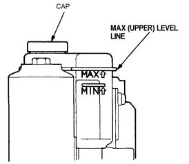
2. Before installing the modulator unit on the car, be sure to bleed the air from the suction port in the modulator unit by leaning the modulator unit to one side slowly (about 45 degrees) as shown.
