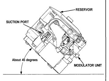
CAUTION: When installing the modulator unit, be careful not to turn it upside-down or lean if excessively.
