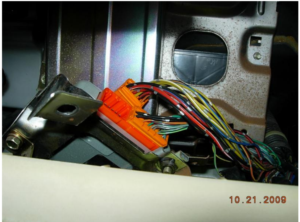
Photo of wires to be disconnected off of module on first bracket that has been unbolted.
