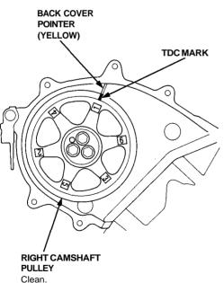
5. Install the timing belt in the sequence shown.
