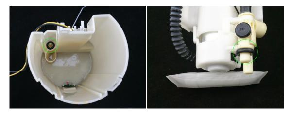
7 - reinstall the center assembly into the bucket assembly and plug in the fuel level sender connector
