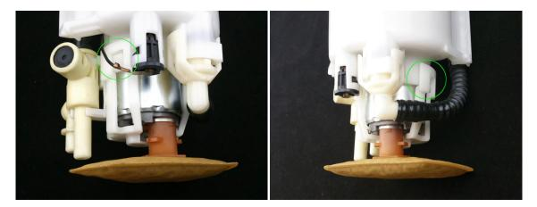
3 – example of the OE pump, fully dressed and the parts that will be removed from the pump and reused on the DW65c/300c
