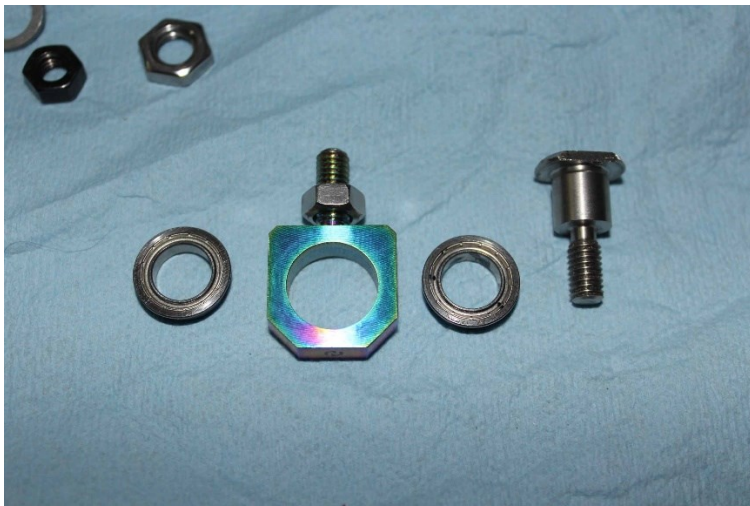
Above, new eyebolt, shoulder bolt and ball bearings for repair. Shoulder bolt head is cut down for clearance and flats ground on the head for a holding wrench. Some thread length was shortened for installation and clearance.
