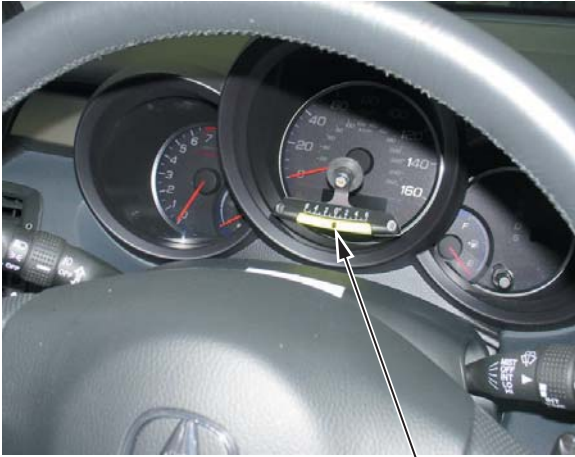
Calibrate the road crown gauge.
