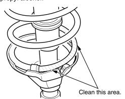
4. Install one half of the spring silencer tube over the second coil about 25 mm (1 inch) past the end of the spring.
