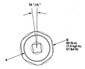
Retighten the rack guide screw to 3.9 N·m (0.4 kgf·m, 4 lbf-ft), then back it off to the specified angle.
