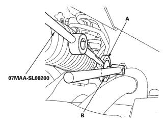
Remove the old sealant from the rack guide screw (A), and apply new sealant (Loctite 565) to the middle of the threads (B). Loosely install the rack guide screw on the steering gearbox.
