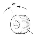
Tighten the rack guide screw to 25 N·m (2.5 kgf·m, 18 lbf·ft), then loosen it.
