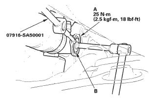
3. Remove the old sealant from rack guide screw threaded section, and apply new sealant around the threads (A). Loosely install the rack guide screw on the steering gearbox.
